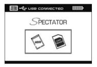
Connect the SPECTATOR to your computer with the USB cable. Then you can select that the device will be identified as an HDD or CARD REARDER. Press  $\Box$  button to confirm your choice.
